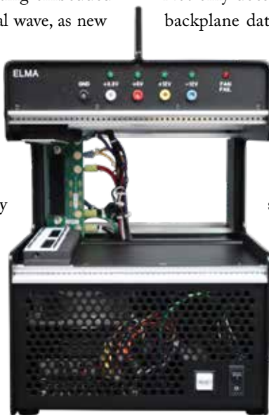
The Elma VITA 48.8 Air Flow-Through development platform, is for developing and testing boards used in air-flow-through systems.
